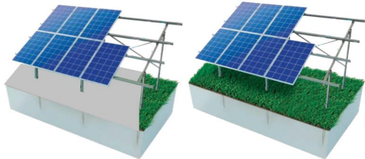
Fig.3. a) Solar array over grass covered ground b) Solar array with a white reflective membrane under the panels
